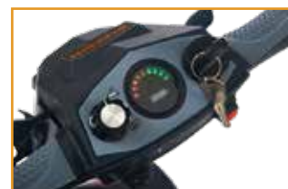
LED battery indicator on the console
