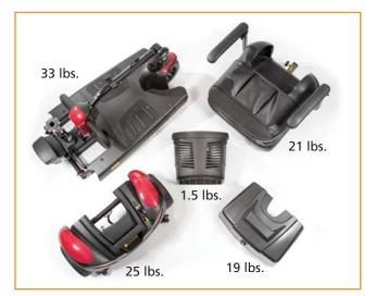
Quickly disassembles into five, lightweight pieces for easy transport!
